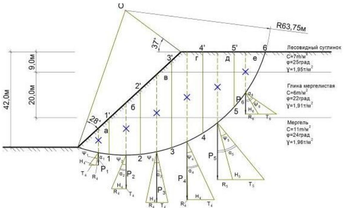
**Figure 2** – Calculation scheme of the surface slope
